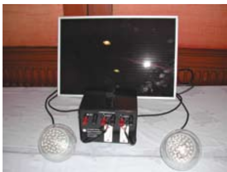
Solar powered 2-lamp LED system
